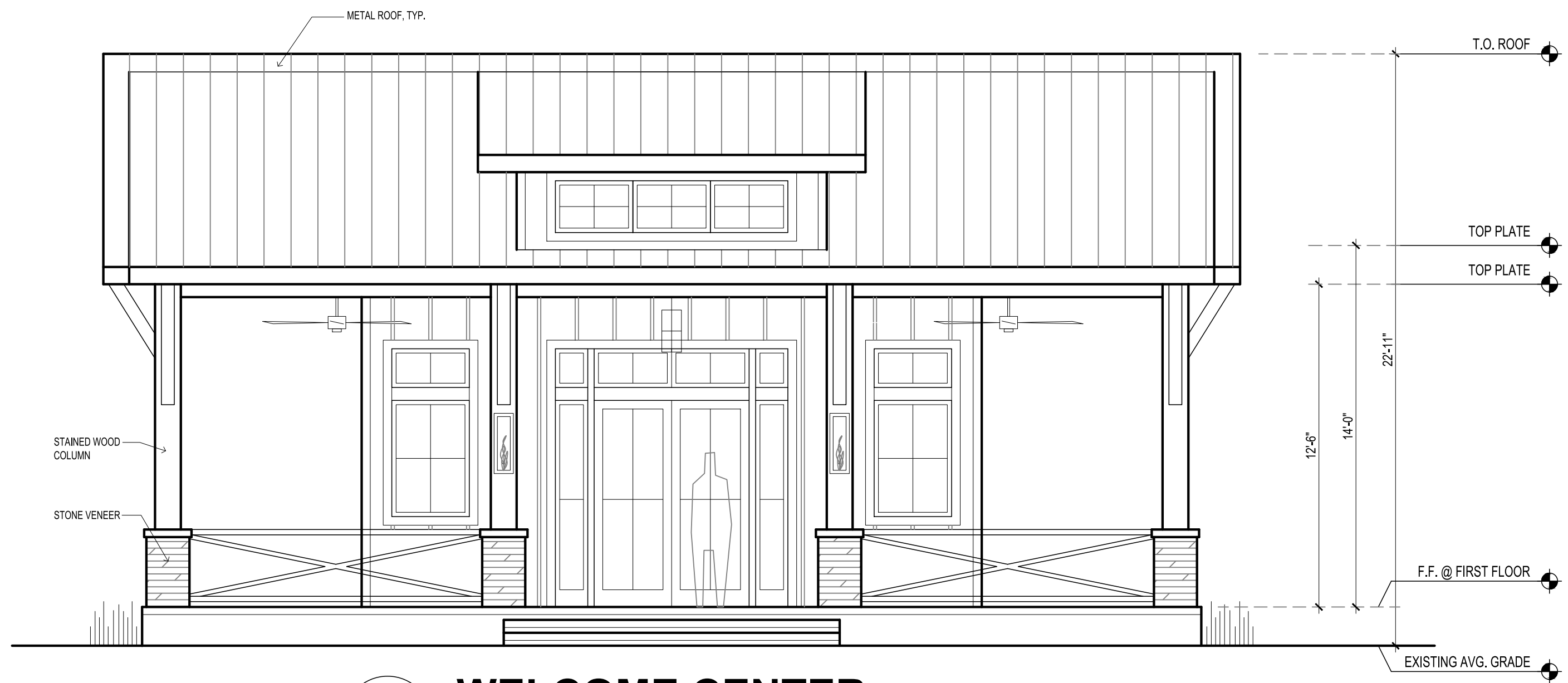
2 WELCOME CENTER 1/4" = 1'-0" FRONT / NORTH ELEVATION
